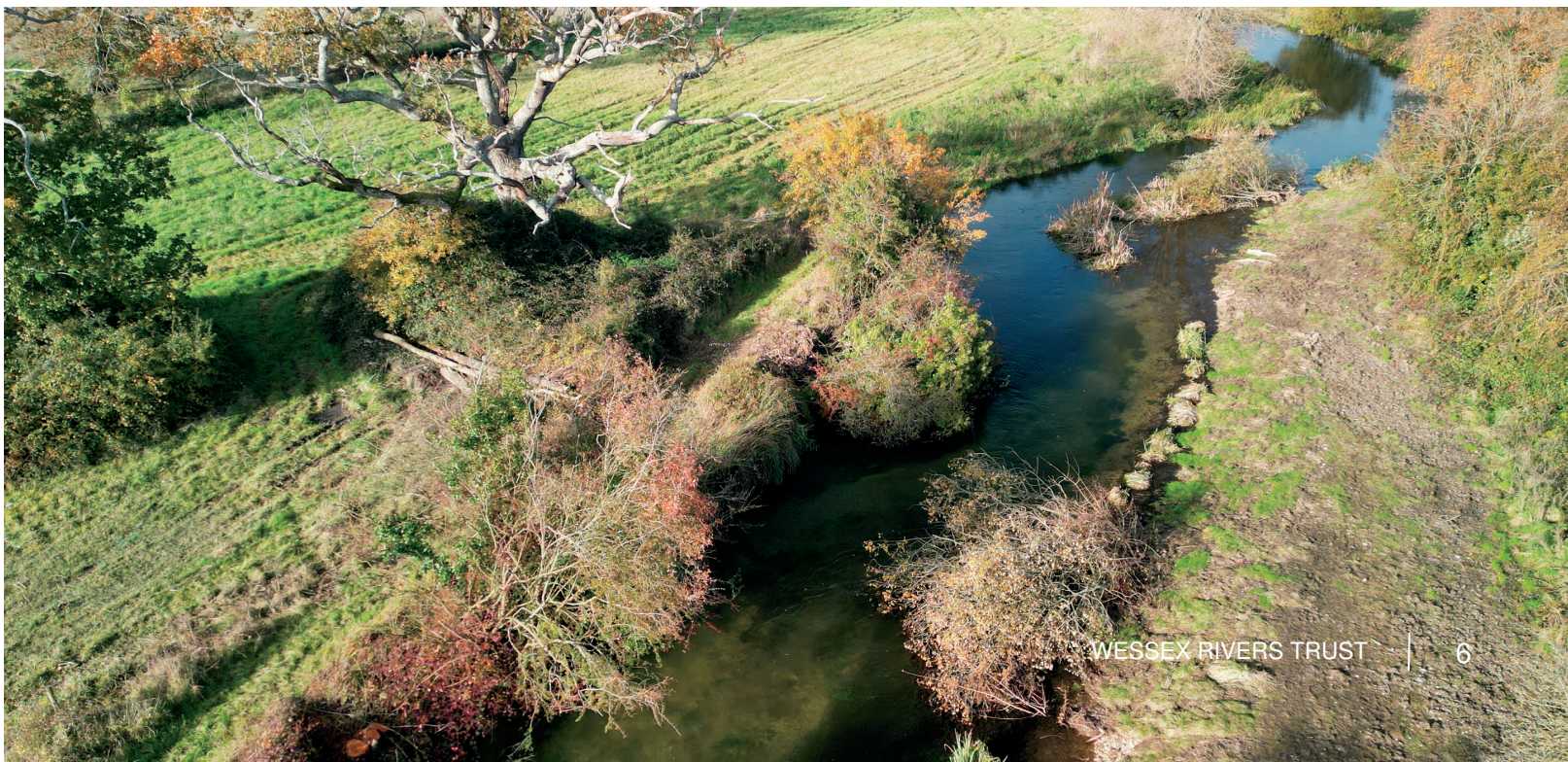
Oakley Bend becomes Oakley Bends. As well as grading down the shear bank, pushing bankside willow and hawthorn into the channel gave this stretch a lovely new meander.
