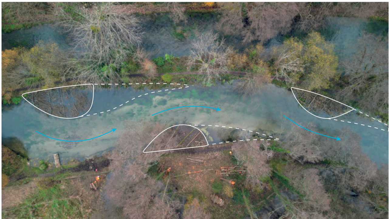
Images 3 & 4 Above: Almost instant scour and sorting of bed gravels resulting from installation of large woody material i.e. 'hinged' trees and coarse woody material i.e. brushwood berms. Dashed blue indicates new scour pools and dashed white areas of marginal deposition.
